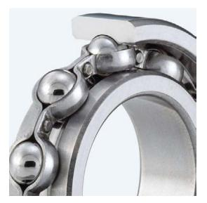
Radial ball bearings have a small initial contact angle of ~ 8° that helps reduce the stress caused by the weight of the load they are supporting.
